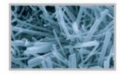
Our Calumex products are based on the ternary system, where alumina, sulphate and calcium are combined to form Hydrated Calcium Aluminum Sulfate Hydroxide or Ettringite crystals.
